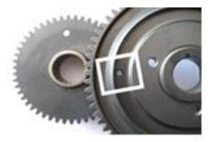
Starter gear: Rotax part nr.: 434 844 see picture below is allowed to be used. Balancing gear: engraved with nr. 635 745 00 see picture below is allowed to be used.
