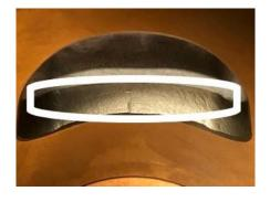
The exhaust port is CNC machined but not over the entire length
