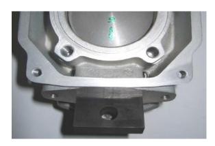
Only the original gasket between cylinder and powervalve house is allowed. Modifications are not allowed.
