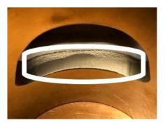
The exhaust port is CNC machined but not over the entire length
