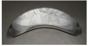
The flange for the exhaust socket may show either cast finish or machined surface. Machined surface can be either flat or show a circular sealing bump.
