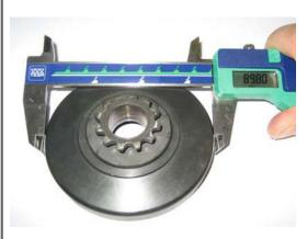
The inner diameter of the clutch drum: maximum 84,90mm. The inner diameter has to be measured with a sliding caliper. The measurement has to be done in the middle of the clutch drum (in the contact area between clutch and clutch drum).
