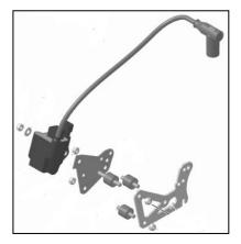
In case the mounting bracket is in conflict with a chassis component, the additions of 2 spaces, one per mounting hole, with a maximum thickness of 20mm between the mounting bracket and the gearbox cover is allowed. Two different mounting versions (left illustrations and right illustration) are legal.
