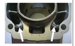
Cylinders with code 613372 the upper edge of the central boost may show factory machining. See picture.
