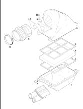
Intake silencer tube (pos2) and carburettor socket (pos 6) are marked with the wording "Rotax".
