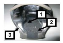
Machined areas are: Top end of piston, outside diameter, groove for the piston ring, bore for the piston pin, inside diameter at bottom end of piston and some pre-existing factory removal (3) of flashing at the cut out of the piston skirt.
