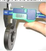
Thickness of the clutch shoe: minimum 24,10mm
