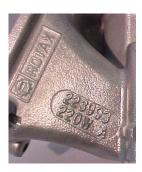
Cylinder types >2018, partnr : 223993 marked with the letter "V" into the inlet port are also allowed.
