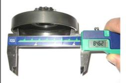
The height of the clutch drum with sprocket: minimum 33,90mm
