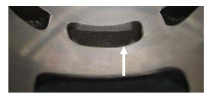
The top edge of the exhaust port may show either just a cast finish surface or signs of a CNC machining or sign of CNC machining in combination with sign of manual grinding.
