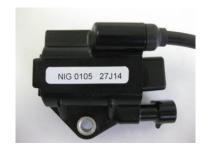
Ignition coil must show two pins at the terminal. The ignition coil is labelled with two stickers: "BRP 666820" and "NIG 0105". The ignition coil is still legal to be used if one or both stickers disappeared.
