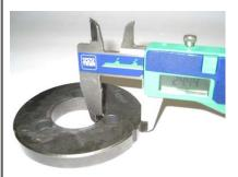
Measurement has to be done at the 3 open ends of the clutch, 5-10mm from the machined groove (all clutch shoes must be completely closed at measurement – no gap)
