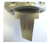
All transfer ports and passages have cast finish surface except some removal (done by the manufacturer) of cast burr at the inlet passage, exhaust port and passages. All ports have chamfered edges to prevent ring snagging. Any additional machining is not permitted. The top edge of exhaust port may show some pre-existing
