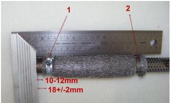
Clamp (1) must be fitted at a distance of 18 (+/-2mm), measured from the end of the tube.
